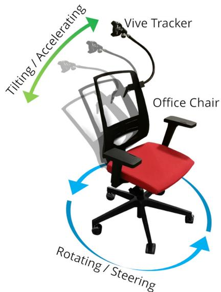
**Figure 2:** The mapping of a regular office chairs' movement onto our VRChairRacer racing cart. An HTC Vive Tracker is used to recognize the chair's position and for accelerating through tilting the back. Rotating the chair is used for steering.
