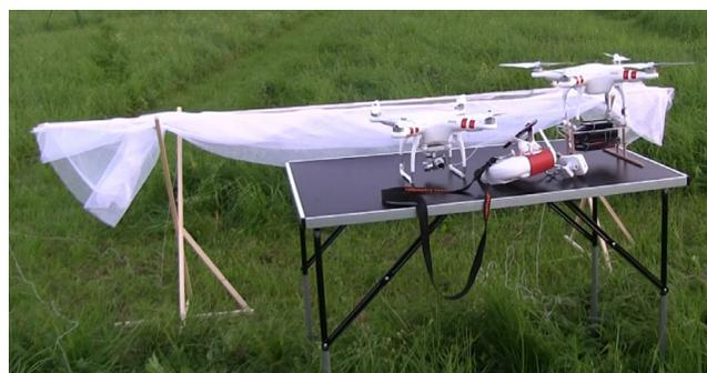
**Figure 2. Drone-based flying display with a mounted canvas and mobilephone with a small built-in projector.**
