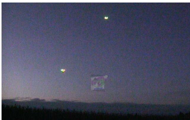
**Figure 4. A Drone is pulling up a 2mx3m canvas and a second drone is hovering close by. The second drone is holding the projector for displaying content on the canvas.**
