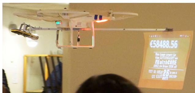
**Figure 1. Drone-based flying display with a mounted canvas and mobilephone with a built-in minibeamer.**
