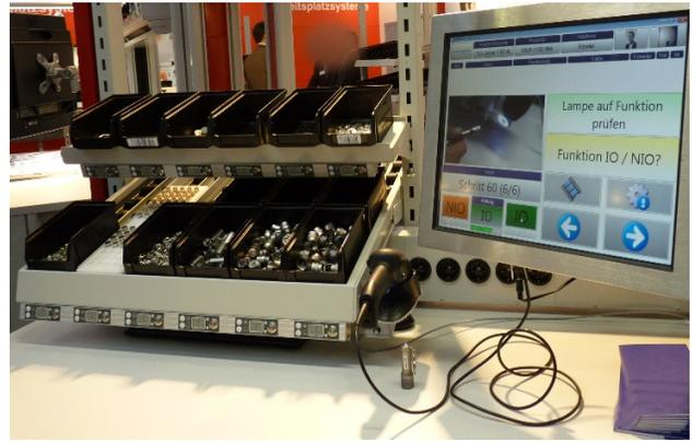
**Figure 2: A workplace-integrated assistive system using a monitor to display instructions for upcoming tasks. The workplace is typical for manual assembly tasks.**
