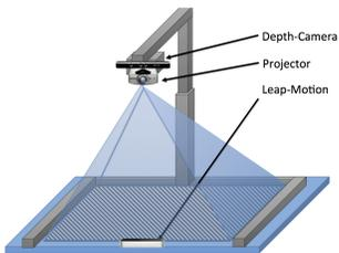
**Figure 2:** An overview about the used technology in our assistive system for the workplace.
