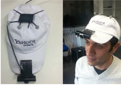
Figure 1. The wearable prototype. The cap includes a webcam for image capture and an OptiTrack marker for exact location tracking
